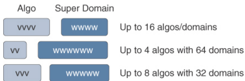
Figure 3-53 SRv6 SID Block Carving (Large-Scale Deployment)
