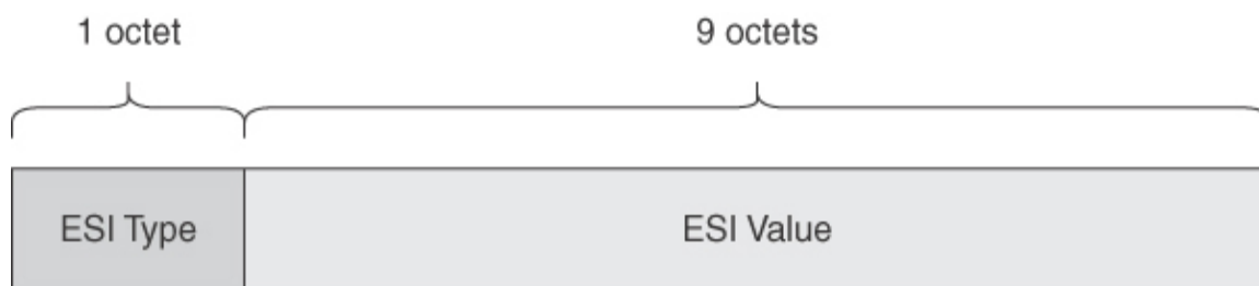
Figure 6-11 EVPN Ethernet Segment Identifier Format
