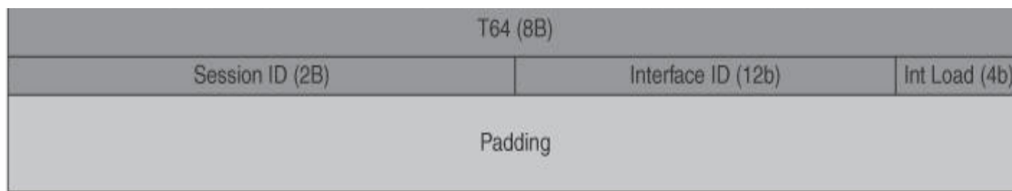
Figure 8-14 Path Tracing Probe Packet Format: Source Node
